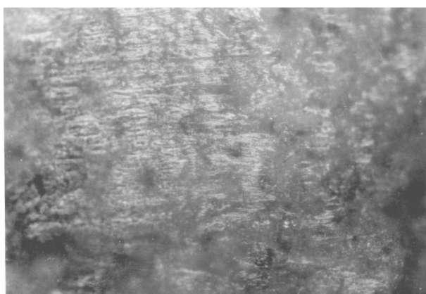
Figure 4 Optical polarising micrograph of a section of injection moulded PP/CaSO 4 -II in the reflection mode.
